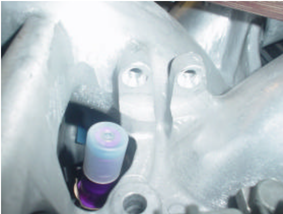
Figure 4 – countersunk bolt holes
