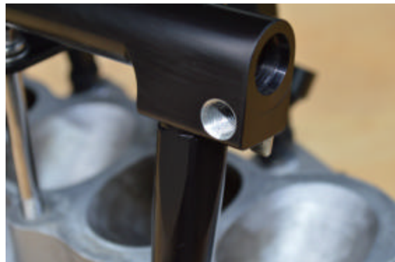
Figure 13 – Fuel temperature sensor boss
