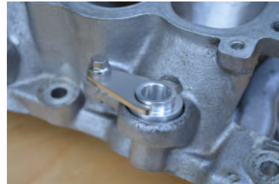
Figure 9 – plenum injector adapter installed
