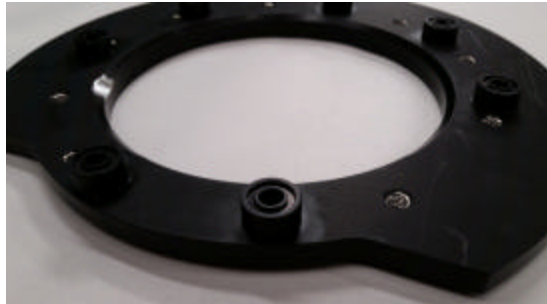
Figure 2 – Adapter back o-ring counter bores
