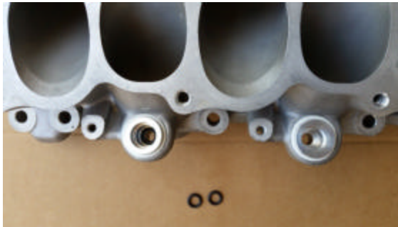
Figure 7 – cushion installed on left
