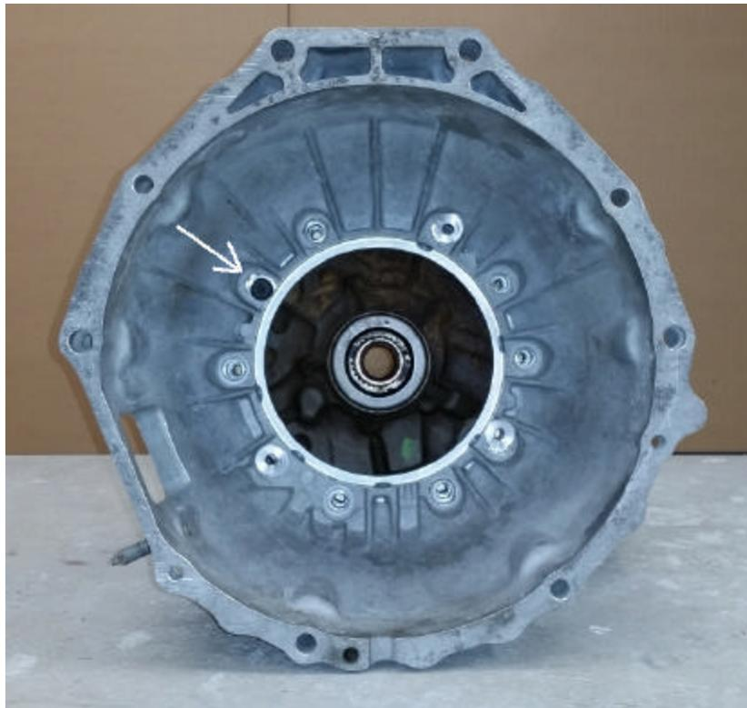
**Figure 7** – VG bellhousing installed, long bolt location
