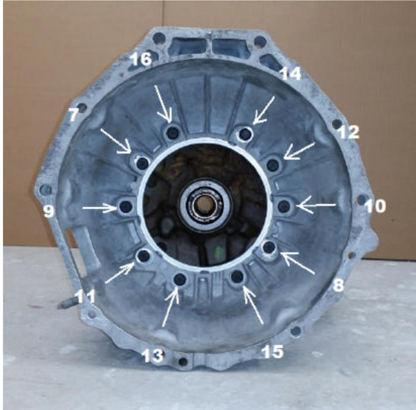
**Figure 8** – bellhousing bolt torque sequence
