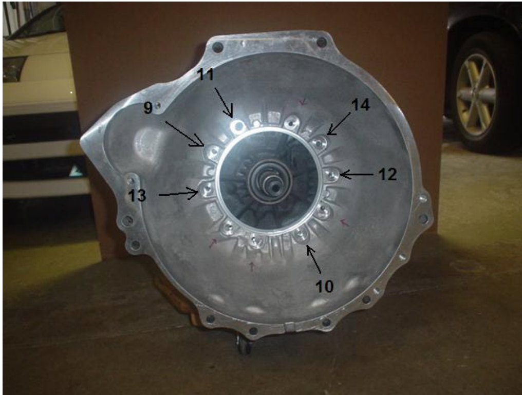
Figure 8 – Short bolt torque sequence
