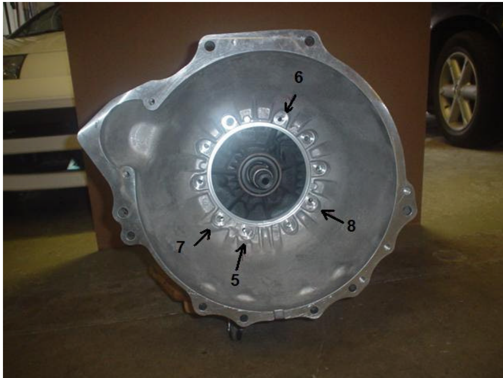
Figure 7 – ZD30 bellhousing installed, long bolt torque sequence
