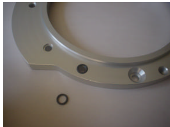
Figure 2 – adapter front o-rings
