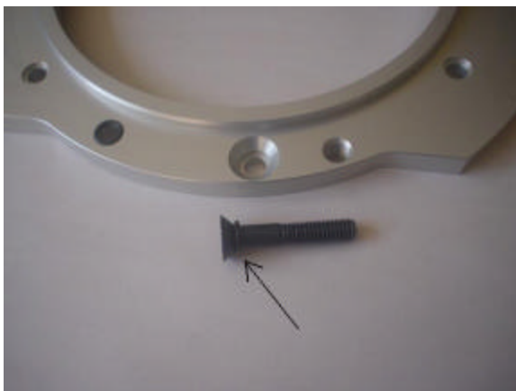
Figure 3 – front o-ring installed on tapered bolt
