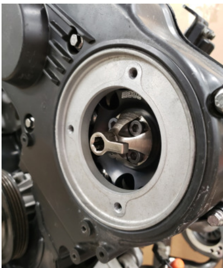
FIGURE 15 - cam sync hub installed
