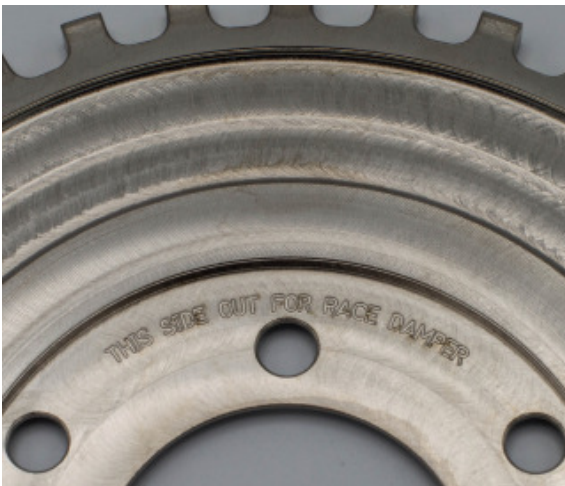
FIGURE 1 - trigger wheel Race damper side out identification FIGURE 2 - PS pulley and trigger wheel bolt holes aligned
