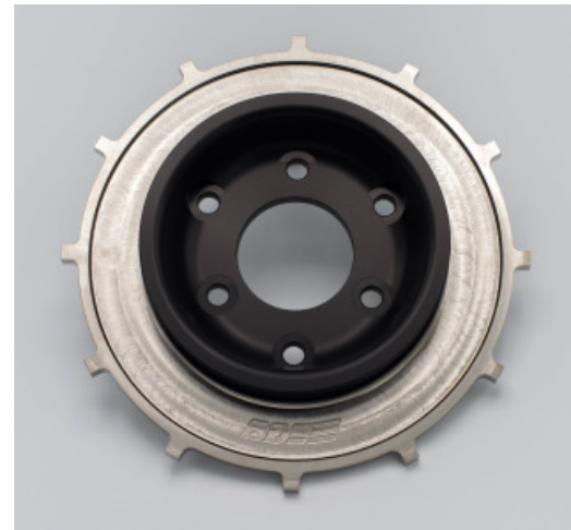
FIGURE 1 - trigger wheel Race damper side out identification FIGURE 2 - PS pulley and trigger wheel bolt holes aligned
