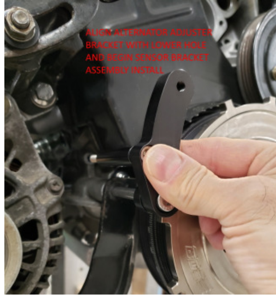
FIGURE 6 - alternator bracket and sensor bracket assembly
