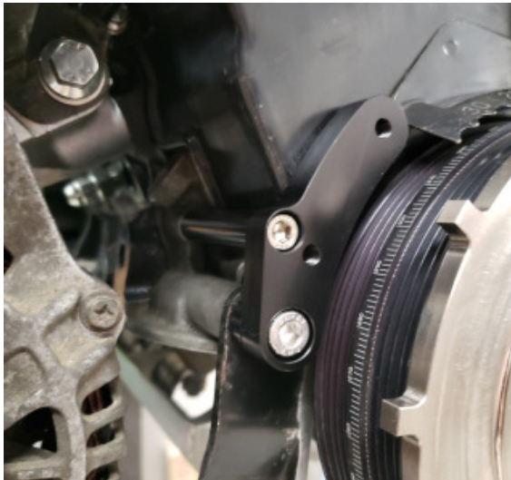
FIGURE 7 - crank sensor assembly with alt adjuster bracket
