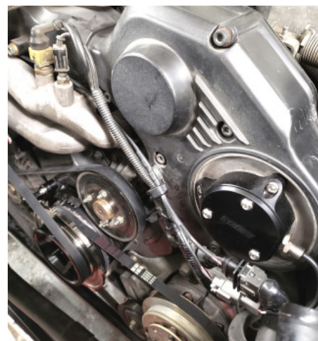
FIGURE 22 - sensor adapter harness installed
