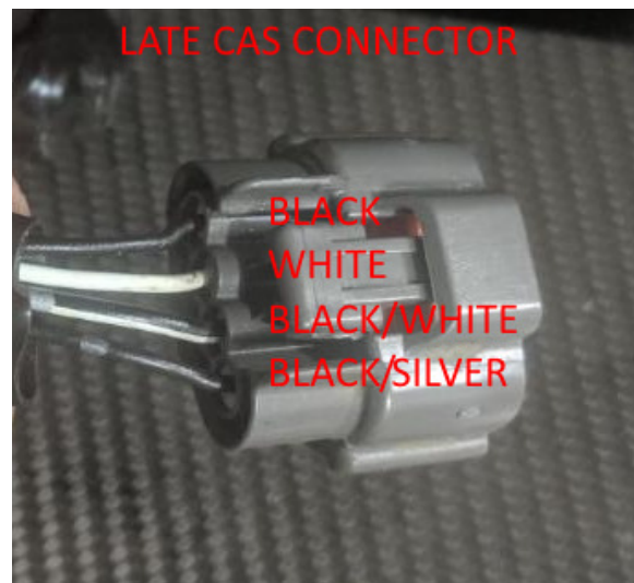
FIGURE 20 - Z32 Late CAS connector wire color orientation
