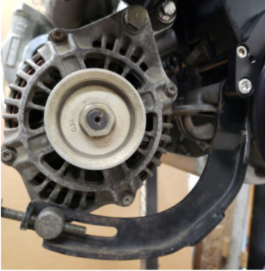
FIGURE 9 - alternator positioned to end of adjustment slot
