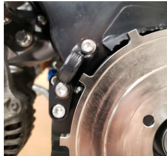
FIGURE 8 - sensor bracket to trigger tooth clearance
