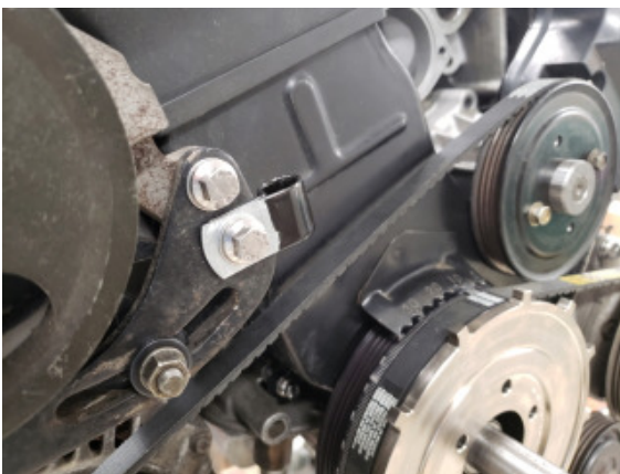
FIGURE 11 - Adel clamp installed on PS mount
