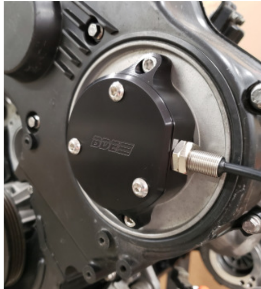
FIGURE 18 - cam sync housing cover installed
