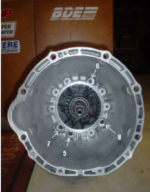
Figure 5 – Long bolt torque sequence
