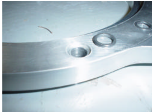
Figure 2 – O-ring counter-bore detail
