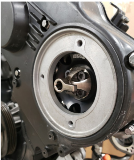
FIGURE 15 - cam sync hub installed
