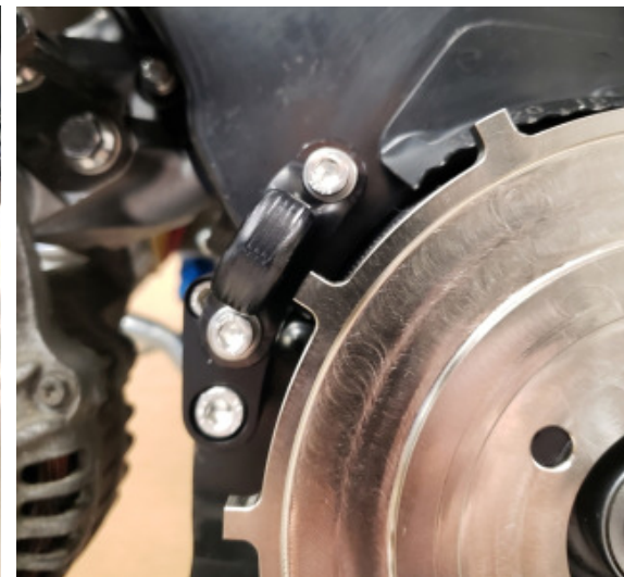
FIGURE 8 - sensor bracket to trigger tooth clearance
