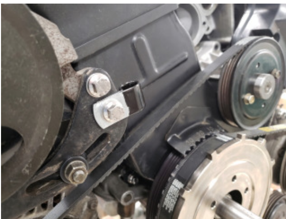
FIGURE 11 - Adel clamp installed on PS mount
