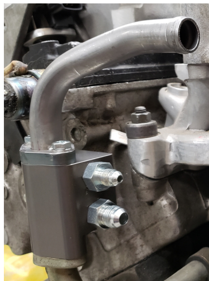
Figure 2 - Low pressure heater pipe assembled
