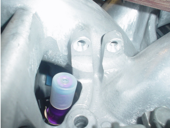
Figure 8 — countersunk bolt holes
