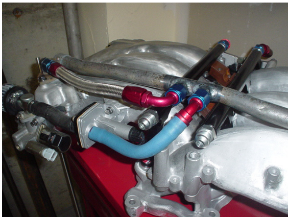
Figure 7 – Idle air plumbed with AN hose fittings
