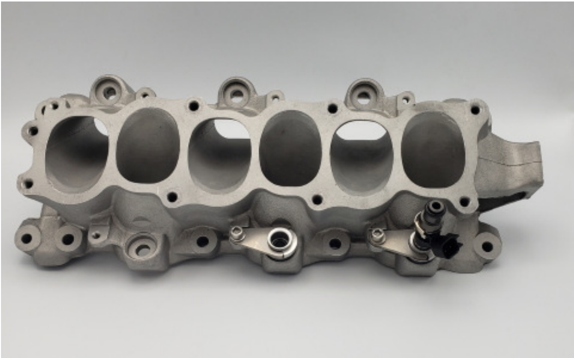
Figure 15 – Late lower plenum injector adapters installed
