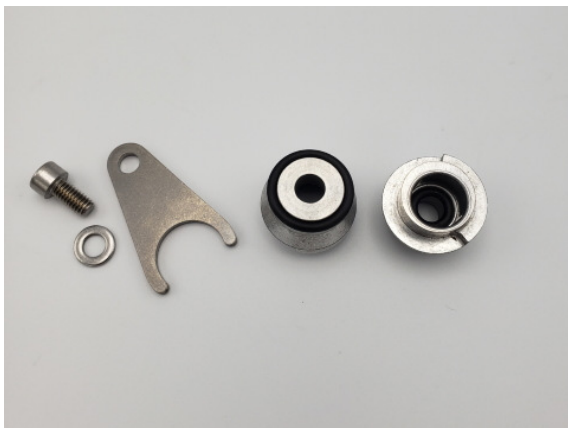
Figure 13 – Late type o-rings installed
