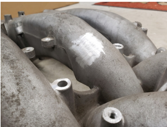
Figure 4 – Early and Late #3 runner boss removed
